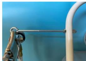
4- To attach the support pole to the dolly, align the two holes on both sides of the U pole with the matching holes on the dolly. Push a screw through from inside of the dolly to the tubes. Use large spacer on top and a small spacer on the bottom between the outer wall of the dolly and the inside of the tube. Secure all four nuts in place on the outside. See (fig 3)
