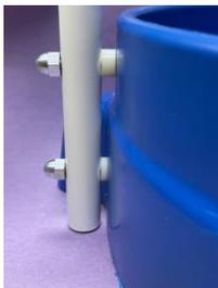
5- Feed the braided suction tube through the large hole in the pump plate so that it will align with the cap of the glue bucket. (fig 4)
