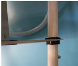
2- Insert support pole through the two outer holes in the pump base plate. Slide it up past the two push locking buttons on the tube (fig 1.)
